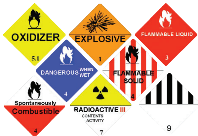
PLACARDS FROM ERG ASSIST IN IDENTIFYING HAZARDOUS SUBSTANCES
